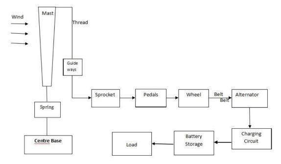
When the wind strikes the mast, it starts to oscillate due to the vortices formed around the structure and suspension spring placed at the bottom of the mast. The energy absorbed by the spring during the oscillation of the mast contributes to the increase in the amplitude of the oscillations. The rib structure with the six thread arrangement at the top of the mast is attached to the bottom chain drives through the guide ways which helps the mast to oscillate in any direction of the wind.
