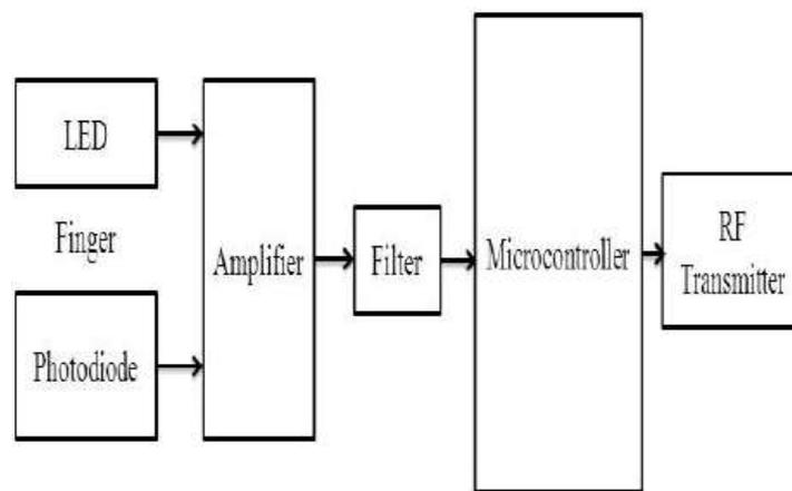
**Fig 3.10: Block Diagram of Heart Beat Sensor**
