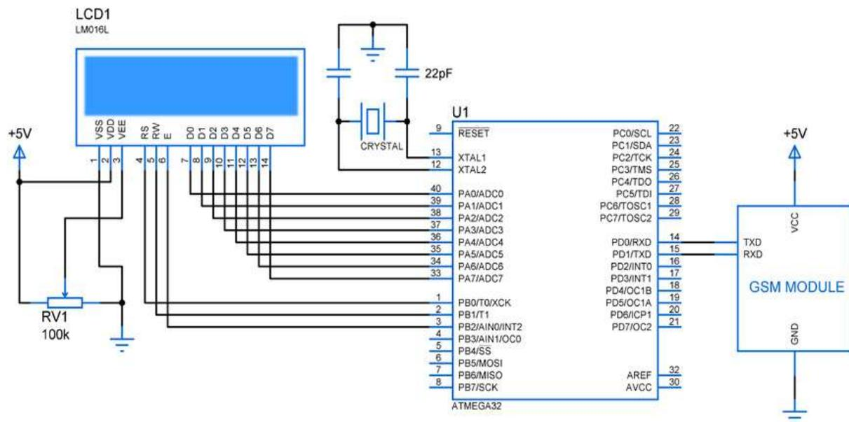
Fig 4.4: Interfacing GSM with Microcontroller
