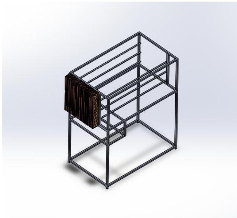
Fig 6: Areca Nut Dryer Frame with the heat exchangers. The three bars on the sides of the frame are where the conveyors will be fixed for drying of areca nuts.
