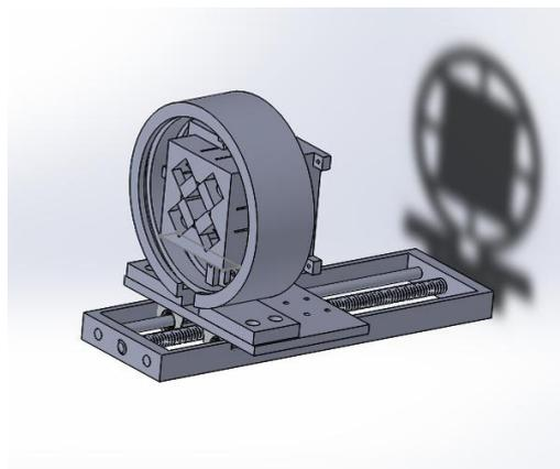
Fig 3 : Design of areca nut holder. (It holds the nut during the process of de-husking and cutting the nut into two.)
