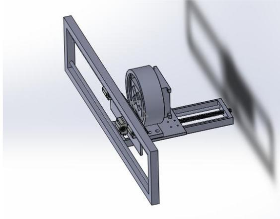
Fig 4: Top view of the areca nut holder in its frame with the cutting blade frame.
