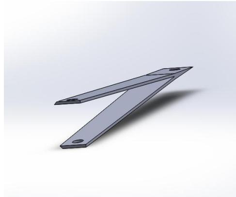
Fig 2: Design of the cutter blade of de-husker.
