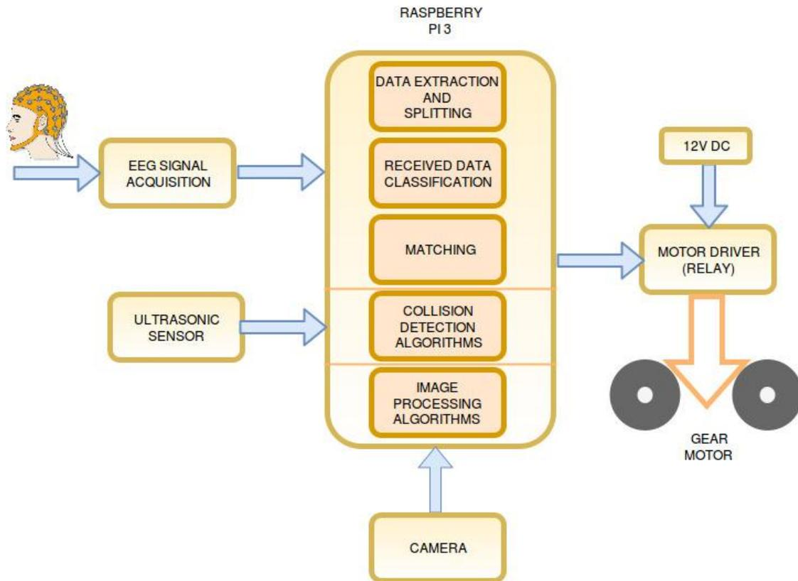
**Figure 1: Basic Block diagram of Brain controlled wheel chair**
