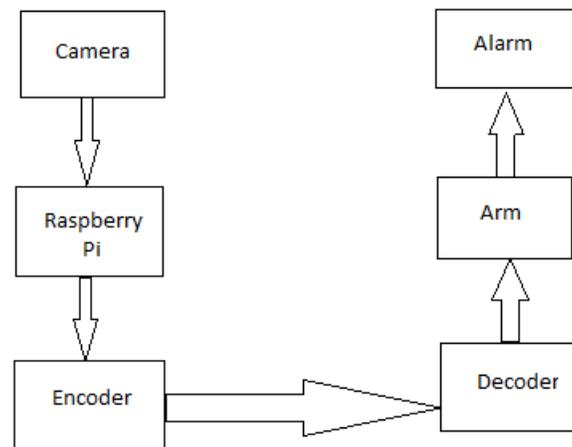
**Figure 2:** System Architecture of Driver Drowsiness Detection System
