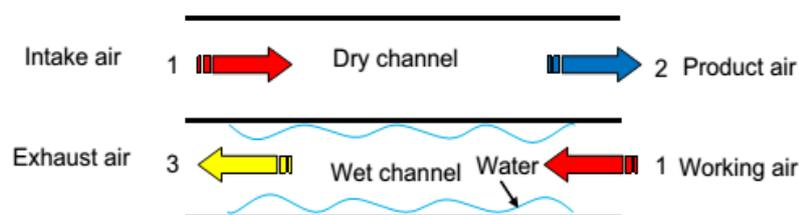
**Fig.3 principle of indirect evaporative cooling**
