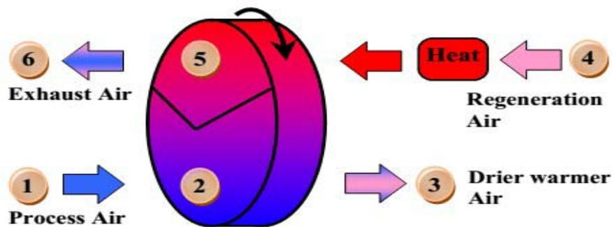
**Fig.4 Principle of desiccant-based dehumidification:**
