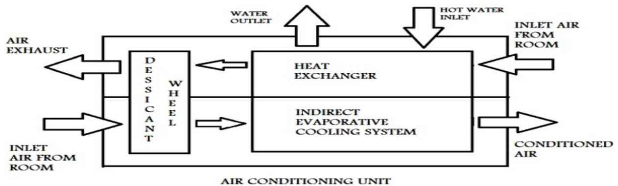
**Fig. 2 Principle of Solar powered evaporative air-conditioning system**
